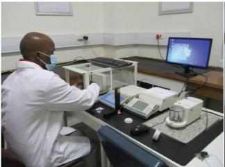
*Image 3: Gravimetric filter weighing in the balance room.*
