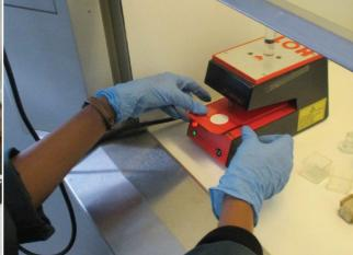
Image 4: Clearing of asbestos filters prior to counting and sizing the fibres.
