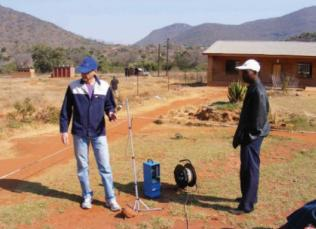
Image 2: An example of a sampling train for conducting environmental asbestos monitoring.
