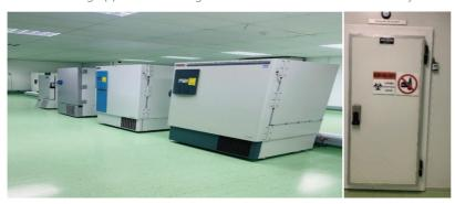
Image 2(A-B): Minus 80 ultra-freezers used for storing samples and COVID-19 vaccines for long-term storage; Minus 20 freezer used for storing vaccines and samples waiting for analysis by the laboratories.
