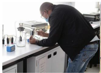
Image 1: Calibration of pumps prior to conducting air monitoring.
