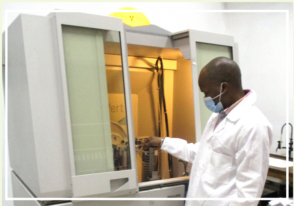
Image 3: Illustration of an XRD instrumentation for RCS analysis
