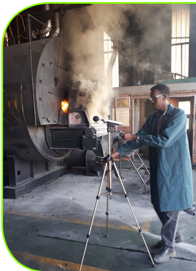
Noise measurements being conducted at the Boiler Room by Ibrahim O' Elimi
