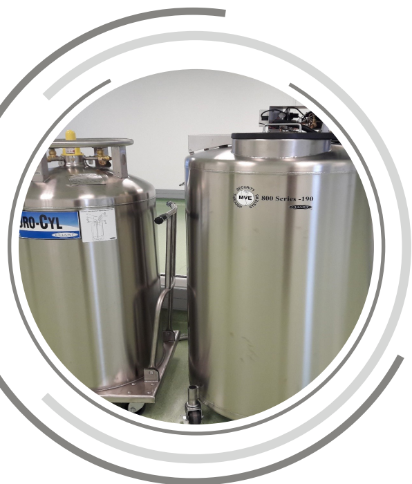
Biobank Liquid Nitrogen tanks store specimen at -156 degree Celsius
