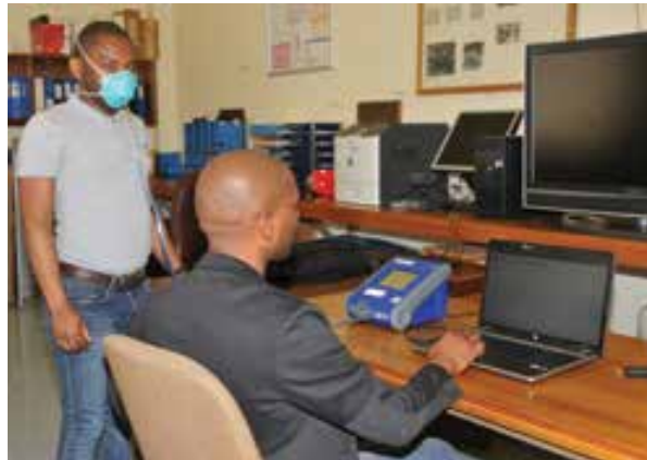
Figure 8: Testing respirator fit using a Portacount
