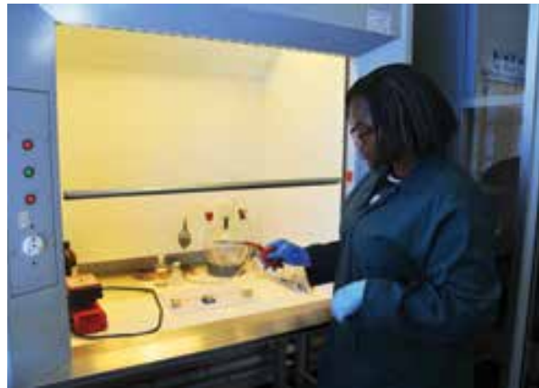
Figure 7: Evaluating airflow direction using a smoke test
